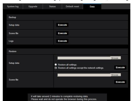
The settings related to backing up or restoring settings data, and saving logs can be configured in this section.
