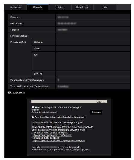
[Model no.], [MAC address], [Serial no.], [Firmware version], [IP address(IPv6)], [Viewer software installation counter], [Time past from the date of manufacture]
