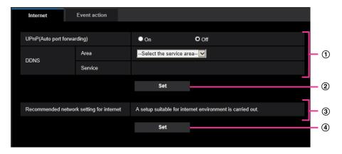
When completing the setting items in field 1, click the [Set] button (②) below field (1). The edited settings in field 1 will not be applied unless the [Set] button (②) below field (1) is clicked. In the same manner as above, click the [Set] button (④) below field 3 when completing the setting items in field 3.
